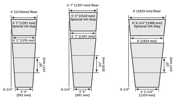
4' x 18" (1219 x 457 mm) Riser = 65-1/4"l (1657 mm) x 20.6"w (523 mm) 4' 7" x 24" (1397 x 610 mm) Riser = 67"l (1702 mm) x 26.8"w (681 mm) 6' x 18" (1829 x 457 mm) Riser = 83-1/4"l (2115 mm)x 20.5"w (521 mm) Optional 4th-Step Must be Removed Prior to Folding for Storage
